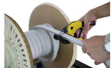
Use recommended cutter to cut the light vertically
