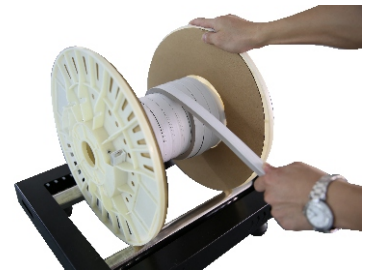
Rotate the roller edge to uncoil the light with another hand
