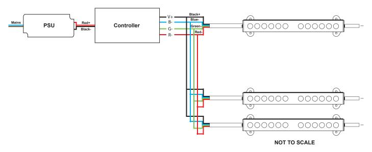
THE MAXIMUM RUN OF UNITS IN SERIES: Regalis I LED Wall washers - 4 x 1200mm / 5 x 900mm / 8 x 600mm / 16 x 300mm Regalis II LED Wall washers - 2 x 1200mm / 2 x 900mm / 4 x 600mm / 8 x 300mm
